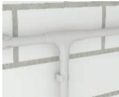
Complete mounting, T piece Mounting is completed after locking on the front section. The T piece can be easily opened again using a screwdriver.
