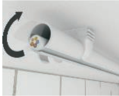
Closing the Quick pipe Turn the Quick pipe in the Quick clip, thus closing the cover.
