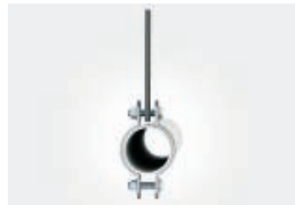
Load 9: Belt end screwed to pipe clamp Minimum breaking load according to column B
