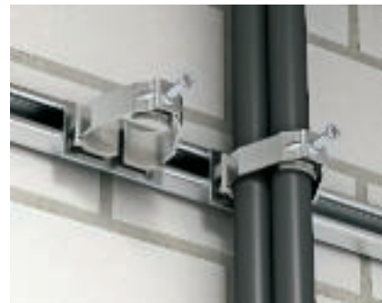
Three single-wire clamp clip The BBS clips 2056/E and 2056U/E are suitable for system routing of single-wire cables in rotary current networks. The arrangement of the external cables remove the magnetic fields, meaning that no excessively high heating need be expected.
