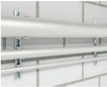
Rail with aluminium Quick clip application The Quick clip is also used in conjunction with rails. This means that the clip can be attached in profile rails with a slot width of 11 mm. This can be used when pipe systems must be mounted on the fastening support "Profile rail".
