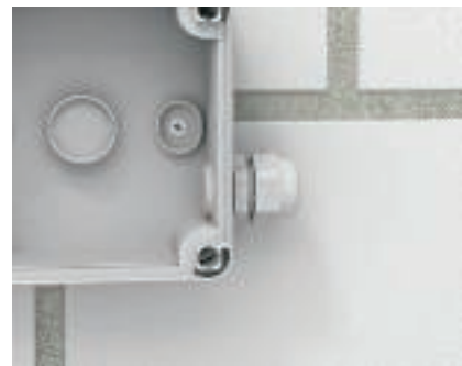
Installation with V-TEC gland The V-TEC cable gland with short connection thread is simply screwed into the available box thread. The soft membrane need not be removed.
