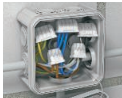
Screwless terminals application in junction boxes Screwless terminals are ideally suited to for wiring cables within junction boxes. Cross-sections of between 0.75 mm 2 and 2.5 mm 2 can be connected in a terminal type using the OBO screwless terminals.
