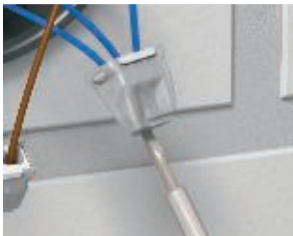
Testing pin opening Practical and safe: the rear testing pin opening allows safe measurement and testing of the wires with a testing pin or phase tester (max. Ø 2 mm).
