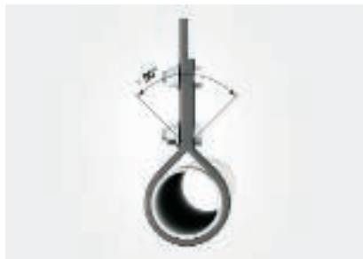
Load 8: Pipe or similar suspended from belt Minimum breaking load according to column A
