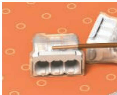
Shortening of wires A mark on the screwless terminal shows the correct amount of insulation to be removed. This not only ensures the perfect fit of the wires, but also maximum touch protection. The correct fit of the wires can be checked through the transparent sight glass.
