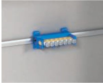
Neutral conductor terminal application Neutral and protective conductor terminals can be snapped onto flat irons, 10 x 2.5 mm, in a lengthwise direction.
