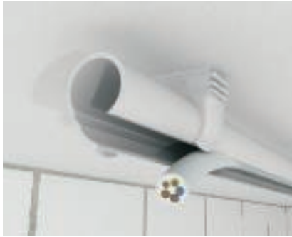
Cable routing in the Quick pipe Insert the installation cable into the opened Quick pipe.
