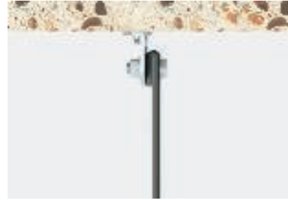
Load 3: Screwed to flat suspender, belt end doubled, free end of belt inside Minimum breaking load according to column A
