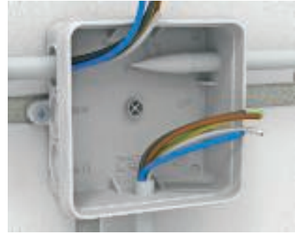
Cable entry, A series The pre-marked cable entries can be opened with a knife or, using the supplied insertion point, directly penetrated with the cable.
