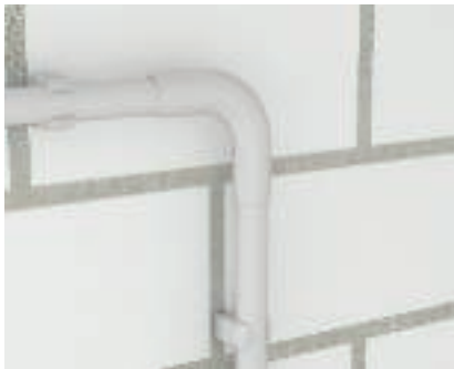
Complete mounting, Quick pipe bend Mounting is completed after locking on the front section. The bend can be easily opened again using a screwdriver.
